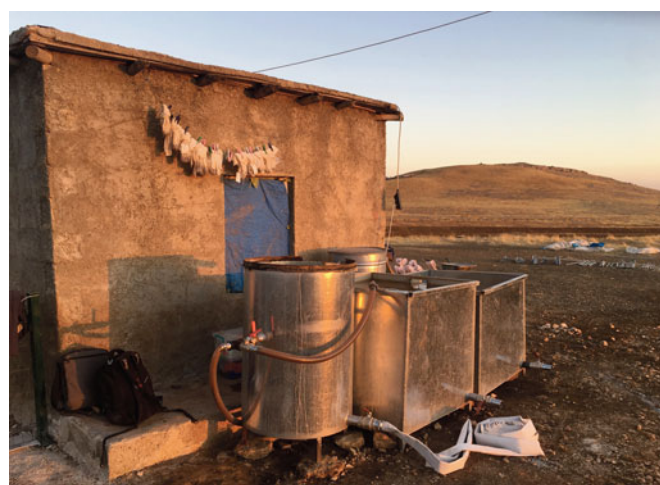
The three-tank, water-recycling flotation system.
