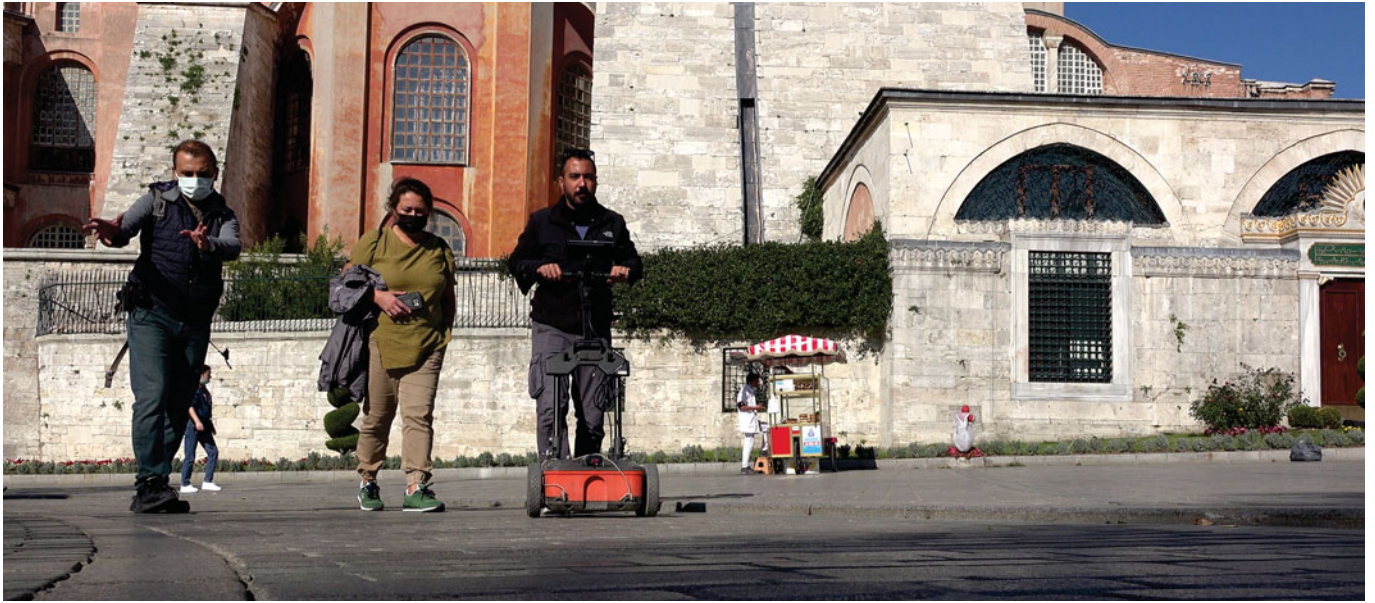
GPR survey work at İshak Paşa Caddesi, east of Hagia Sophia (photograph by Engin Aygün).
